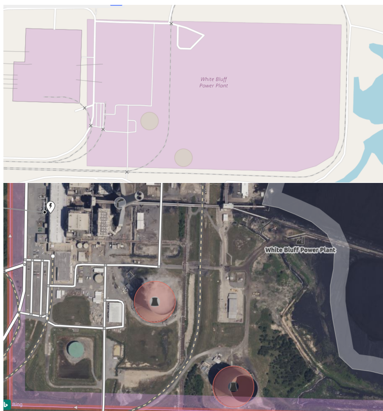
Figure A1. White Bluff power station as shown on OpenStreetMap (top) and in OpenStreetMap edit mode (bottom). We used this aerial imagery to annotate locations of FGD flue stacks (translucent white circle) and NDT cooling towers (red circles).
