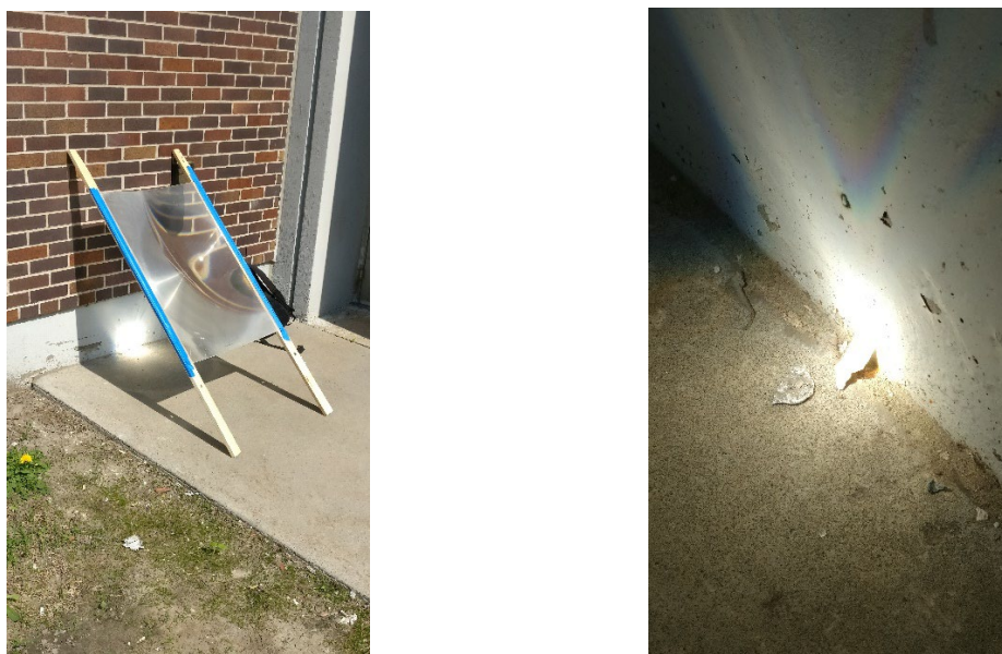
Figure 2. (A) 1 m 2 Fresnel lens solar concentrator capable of attaining ~800°C sufficient to (B) melt aluminium chips under modest solar cover.
