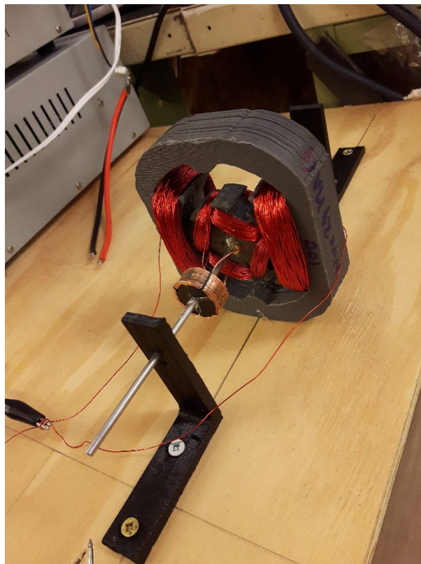
Figure 5. DC electric motors with 3D printed stator and rotor electromagnets.
