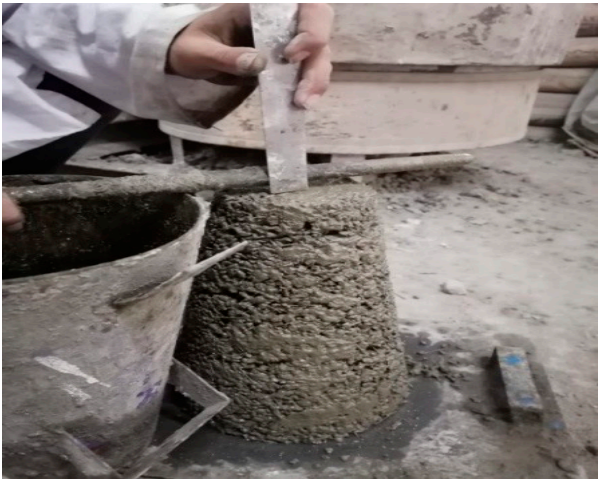
Slump Test on Concrete
