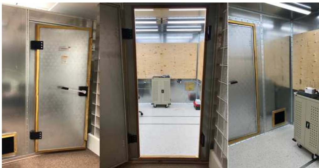
Figure 4. CIC's Faraday Cage used in Bluetooth experiments to block external signals that may interfere with the network traffic collected.
