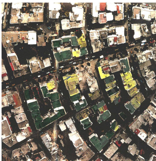
Figure 1. Application of Rapid Visual Screening in a specific area. Samples of structures across the damage spectrum were drawn, to mitigate local effects. The image is courtesy of [16].
