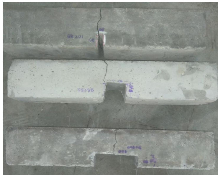
(f) flexural failure behaviour of notch repaired beam.
