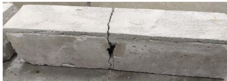
(e) One-point load flexural test on beam specimen.
