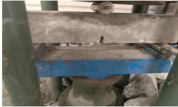
(e) One-point load flexural test on beam specimen.
