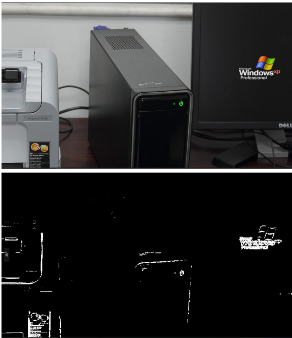
Figure 3. Example of the results obtained after performing the DWT method ( top ) Image with the windows logo and power button manipulated ( bottom ) Results of the DWT based method where sharp pixel variations are enhanced
