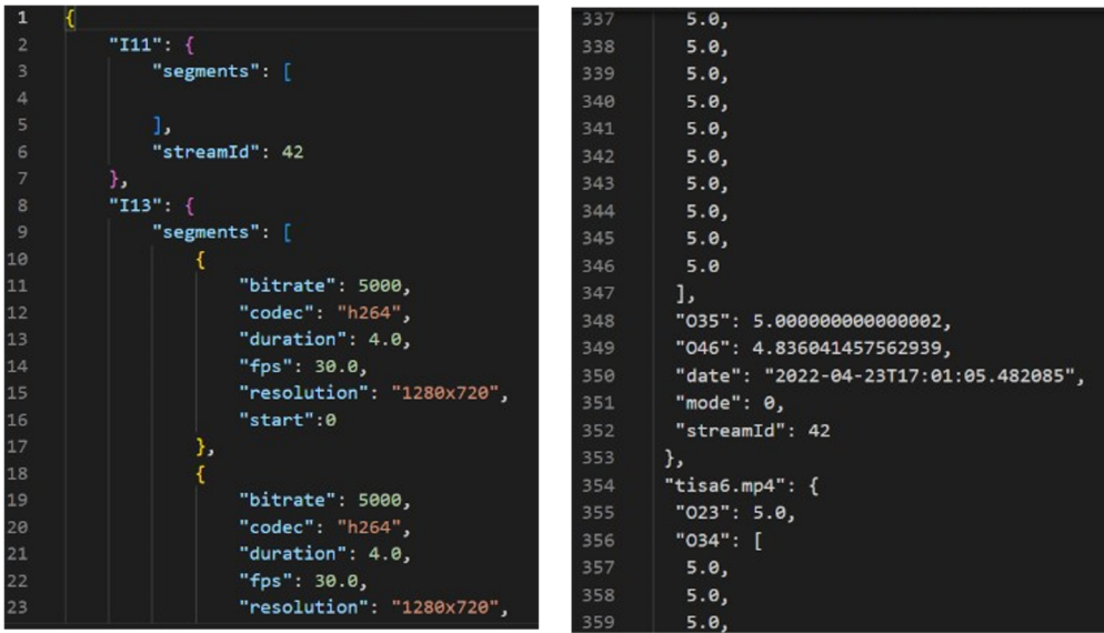
Figure 5. The screenshot of input and output *.json file from ITU-T P.1203. in the left is the input and the right is the output file.
