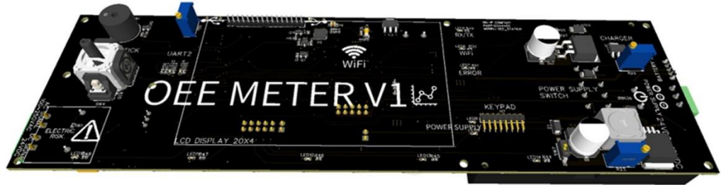
Figure 13. 3D view of the transmitter's PCB (printed circuit board).
