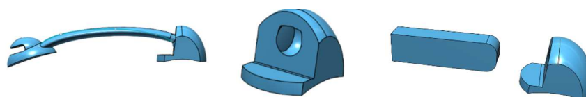
Figure 6. With the arm 1.1 time enlarged prepare the cutout in the molar pad. Then make a cutout to allow the rotation of the arm in the molar pad.
