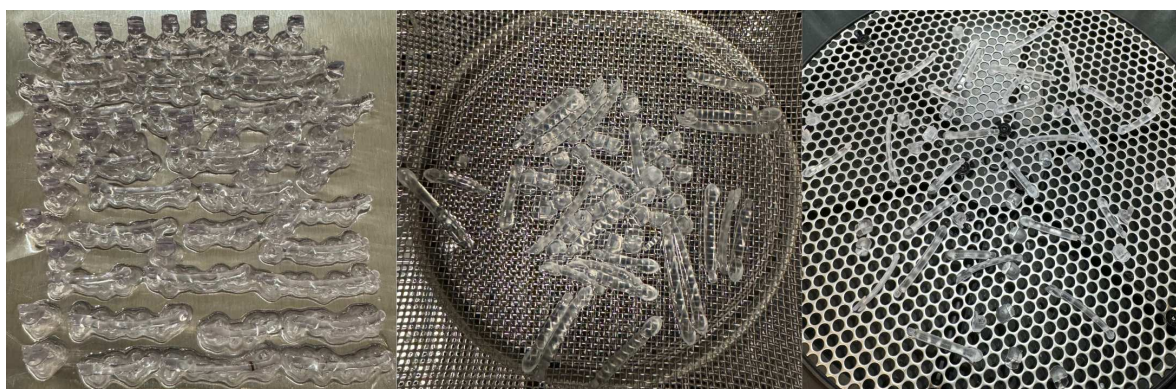
Figure 7. The distalizers on the print plate; the distalizers in the washer; the distalizers after post cure.
