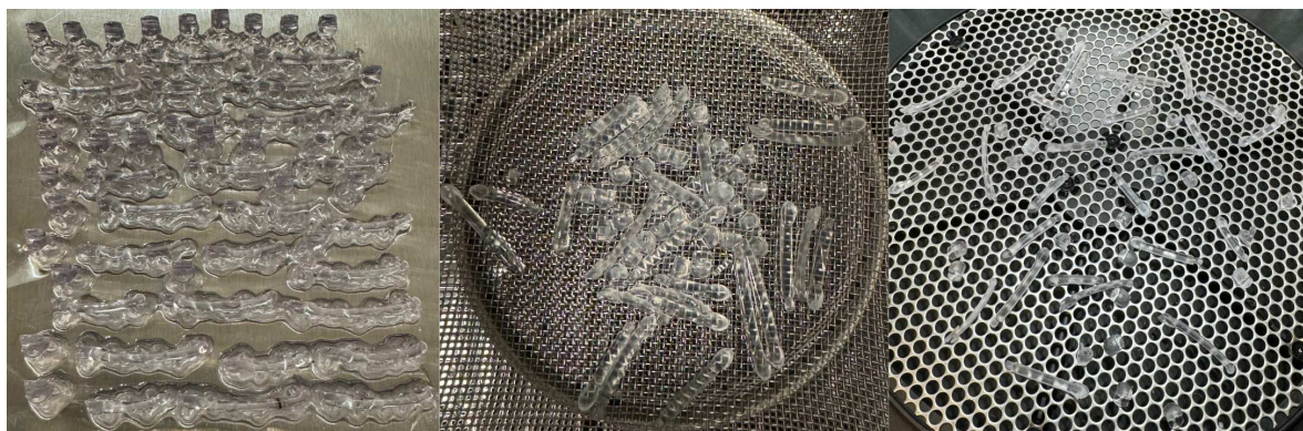
Figure 8. The distalizers on the print plate; the distalizers in the washer; the distalizers after post cure.
