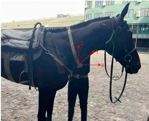
Figure 6. On-site data acquisition using a wearable device placed on the neck of the horse.
