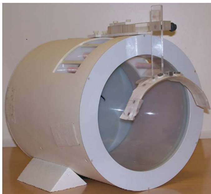
Figure 2. A subject-friendly passive shim system positioned onto the RF coil.
