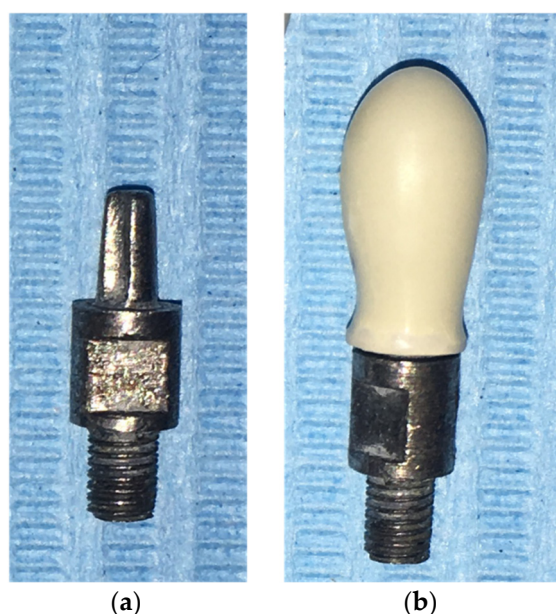
Figure 2. (a) Pin simulating the implant-abutment system provided with a groove that matches with the sample crown; (b) PEKK crown inserted onto the pin.
