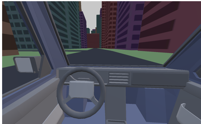
Figure 5. Cars are simple to make rendering computationally inexpensive, including the ego vehicle, which can be adapted to the needs of any specific experiment.
