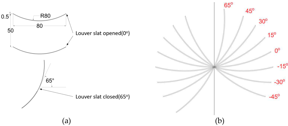
Figure 2. (a) Structure of louver and (b) definition of louver angles used in this study.
