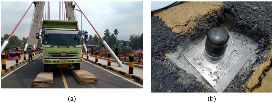
Figure 12. (a) The execution of dynamic load test; (b) The placement of accelerometer.
