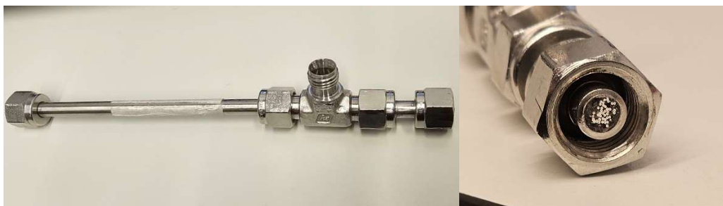
Figure 3. A membrane module for the study of gas transport characteristics of hollow-fibre gas separation membranes.
