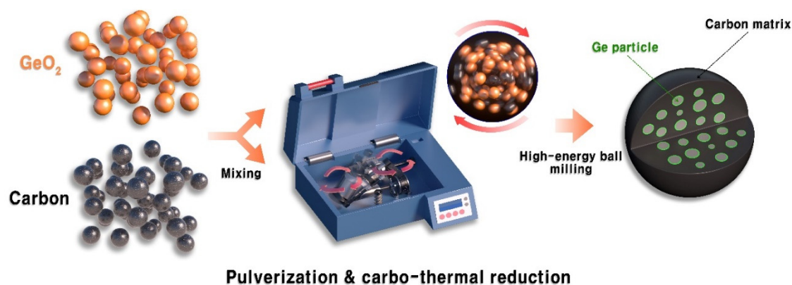
Figure 1. Schematic illustration of high-energy ball milling for synthesis of the Ge@GeO 2 -C composite material.
