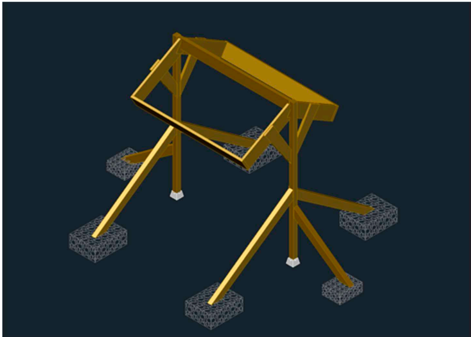
Figure 2. Inverse Y Ballast System.
