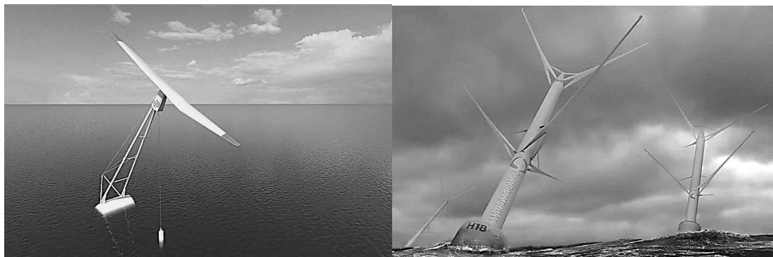
Figure 8. Innovative adaptive floating turbines: on the left is a turbine with a solid inclined rotor [1]; on the right – counter-rotation turbine [2].
