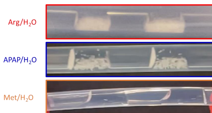
Figure 10. Images of slugs during the crystallization process for Arg/H 2 O (red), APAP/H 2 O (blue) and Met/H 2 O (orange) recorded at a tubing length of L_{tubing} = 12 \text{ m} at Q_{tot} = 20 \text{ mL min}^{-1} . Videos of slugs during the crystallization process can be seen in the supporting information.
