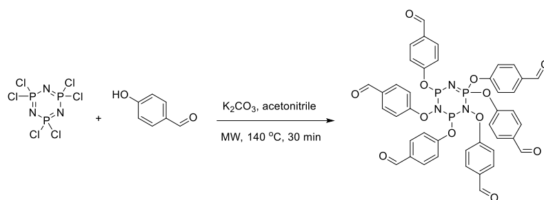
Scheme S3. Synthesis of hexa(4-formyl-phenoxy)cyclotriphosphazene
