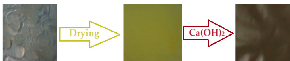
Figure 2. Preparation of sPEEK-M membranes from PEEK solution in sulfuric acid.
