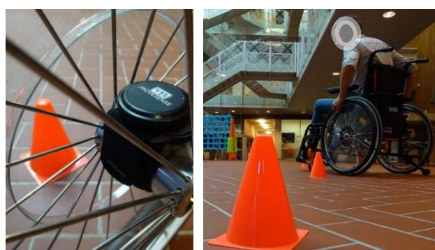
Figure 1. Mounted Movesense sensor and example of the test track.
