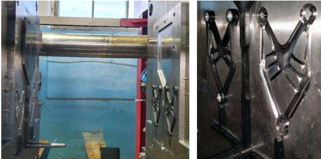
Figure 16. TVA and TVI brackets manufacturing process on an injection molding machine.
