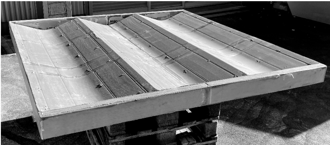
Figure 19. TRC element with geometry G1.0 but half overall height after demolding (lying upside down), Photo: Iurii Vakaliuk.
