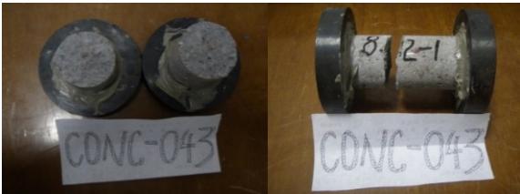
Figure 2. Failure under tensile stress.
