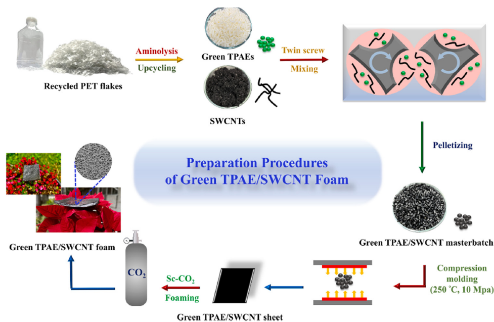
Figure 2. Procedure for preparing green TPAE-SWCNT nanocomposite foams [12]. Copyright 2023, Elsevier.
