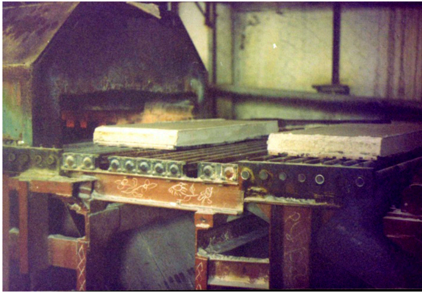
Figure 13. The pilot-scale production of heat insulating boards using expanded perlite.
