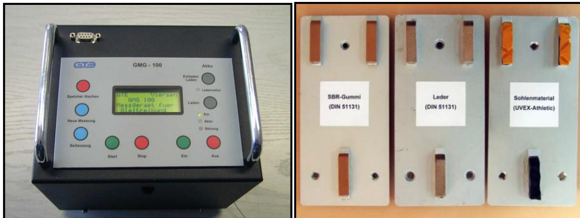
Figure 1. GMG 200 tester and measuring apparatus.
