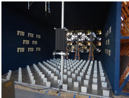
(a) Fully-open vertical spires and ground plates.
