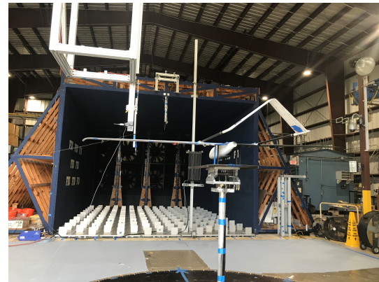
(b) UAV mounted on the test tower facing the oncoming flow.
