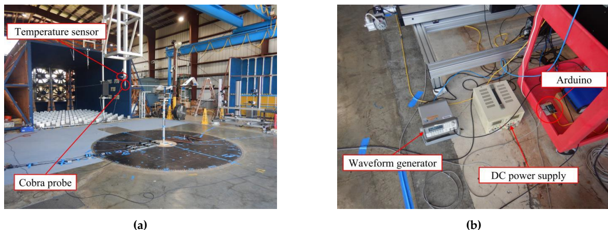
Figure 4. (a) Temperature sensor and additional cobra probe near the UAV (suspended from gantry crane) and (b) Servo control and data synchronization hardware.
