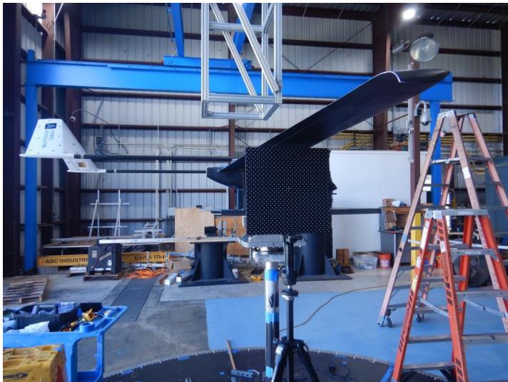
Figure 13. Side-view of the UAV setup during the PIV calibration process.
