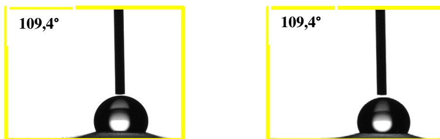
Figure 1. Electrode wetting angles of the electrodes made of AX and YP-50F, besides the Aquivion membrane versus \text{Na}_2\text{SO}_4 and \text{Li}_2\text{SO}_4 (both 1M).
