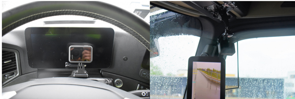
Figure 6. Mounting action cameras to record instrument cluster display and mirror fields of view.
