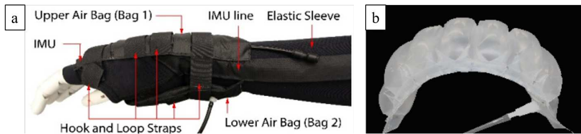
Figure 11. Soft wrist exoskeleton designed by [34] to alleviate CTS: a) the whole device; b) the airbag actuators.
