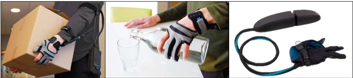
Figure 23. Bioservo Carbonhand® device and examples of related applications [35].
