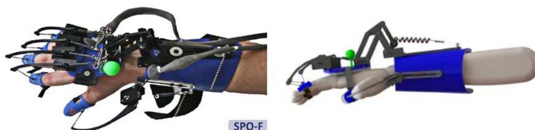
Figure 15. SCRIPT passive orthosis. The SPO-F design developed by [28].
