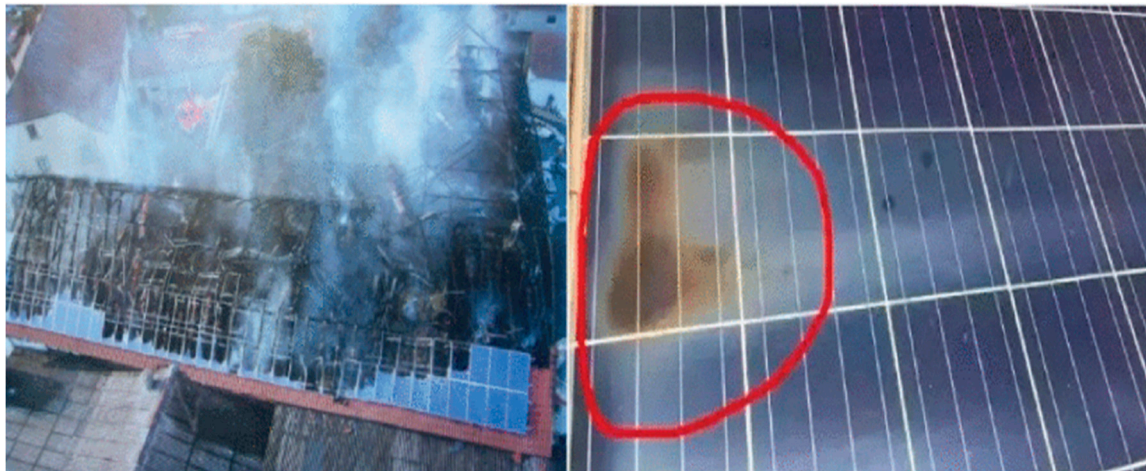
Figure 2. Fire incident in PV array initiated by hotspot failure [30].
