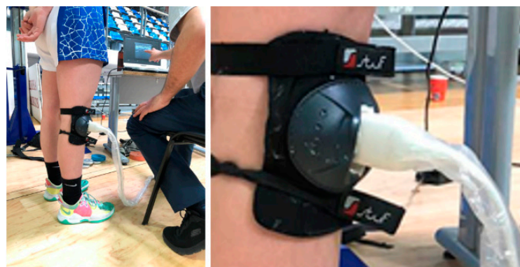
Figure 4. Experimental setup in stage 3 with ultrasound transducer muff for immobility of the transducer regarding the knee joint.
