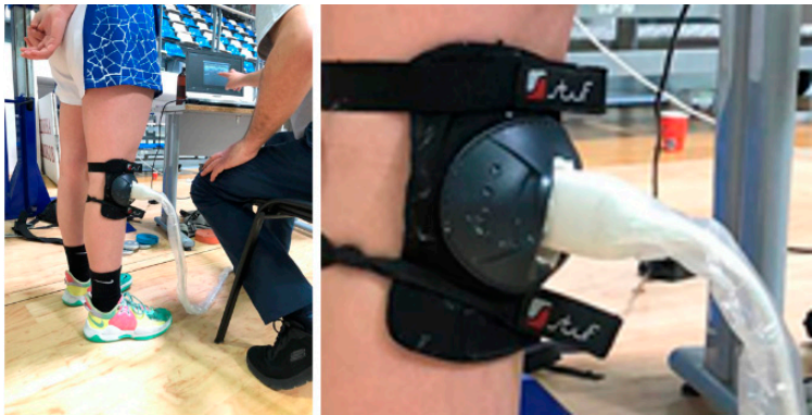
Figure Experimental setup in stage 3 with ultrasound transducer muff for immobility of the transducer regarding the knee joint.
