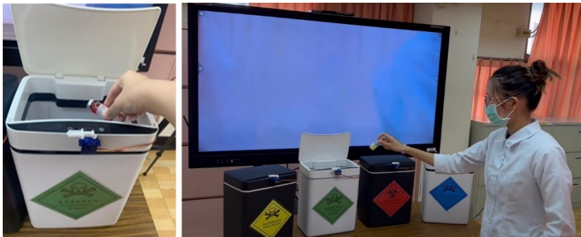
Figure 4. The synchronous system opens the lid of the correct trash and closes once the waste is placed inside. .
