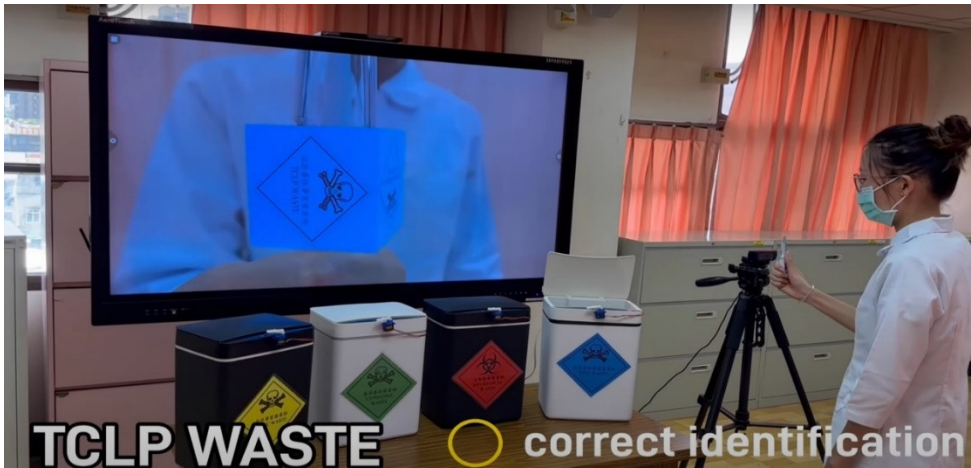
Figure 6. Scan the medical waste classification mark on the medical waste. After the identification is completed, the correct trash can lid of the classified medical waste (this diagram shows biomedical waste) will automatically open.
