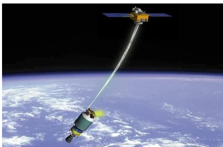
Figure 1. A method for removing space debris using a space tug and a tether system.
