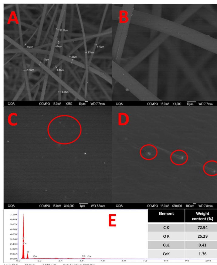
Figure 6. SEM images for the NWF of PET/CuNP (0.5% w/w) sample at different magnifications. A) 350X, B) 1000X, C) 10,000X and D) 30,000X.
