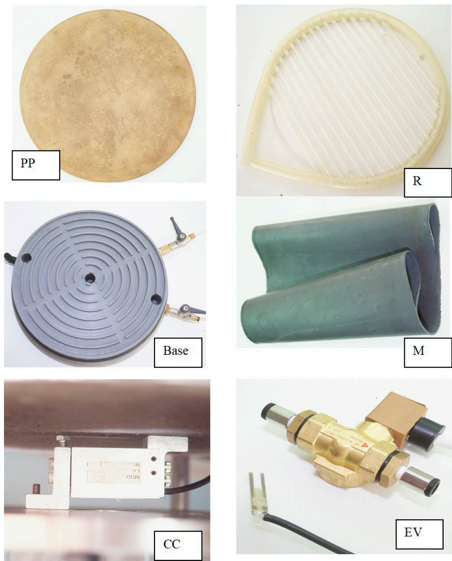
Figure 2. Main components of the column for the study of the hydromechanical properties of the residue. PP: porous plate; R: device for applying the uniformly distributed water recharge; Base: support of the solid and methacrylate column wit sensors, on which the porous plate rests and allows water evacuation; M: latex membrane; CC: load cell; EV: solenoid valve. See main features and details of its functions in Table 1 and [3].
