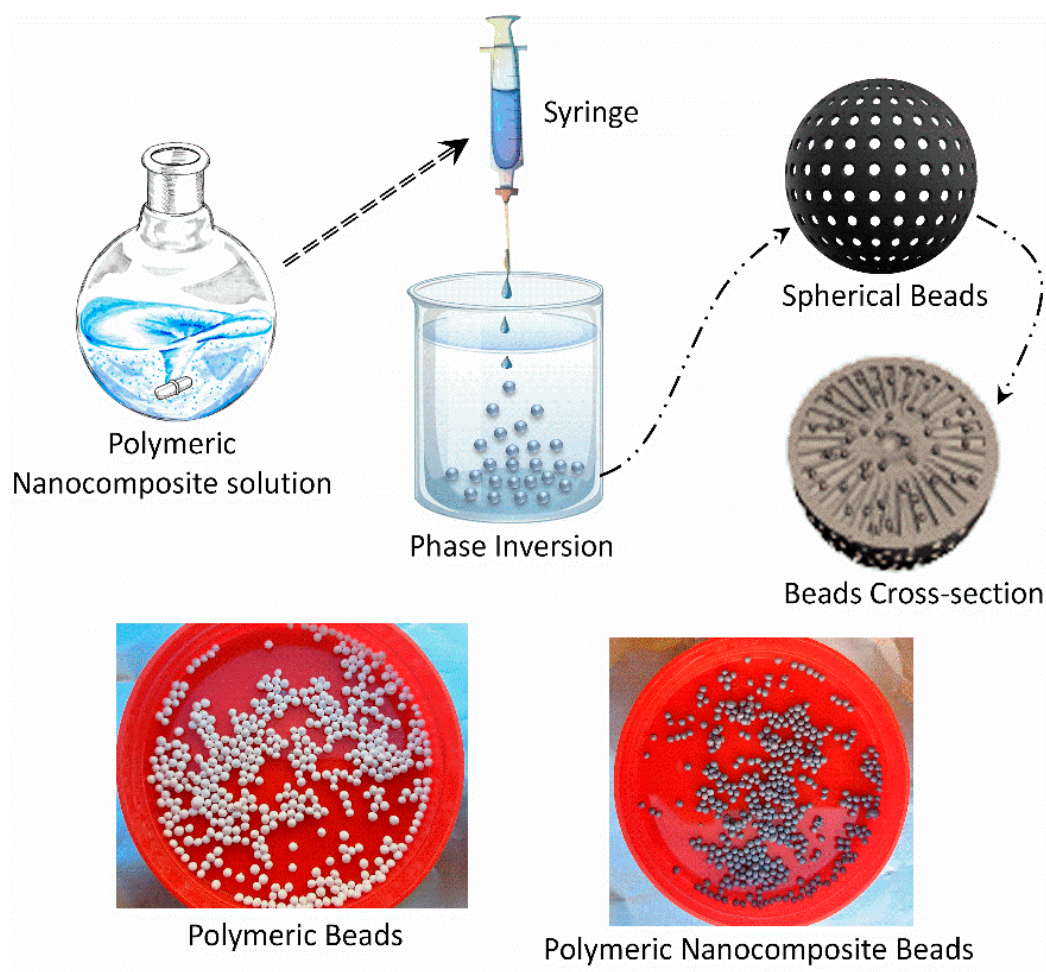
Figure 1. Schematic diagram illustrating the preparation of polymeric nanocomposite beads.
