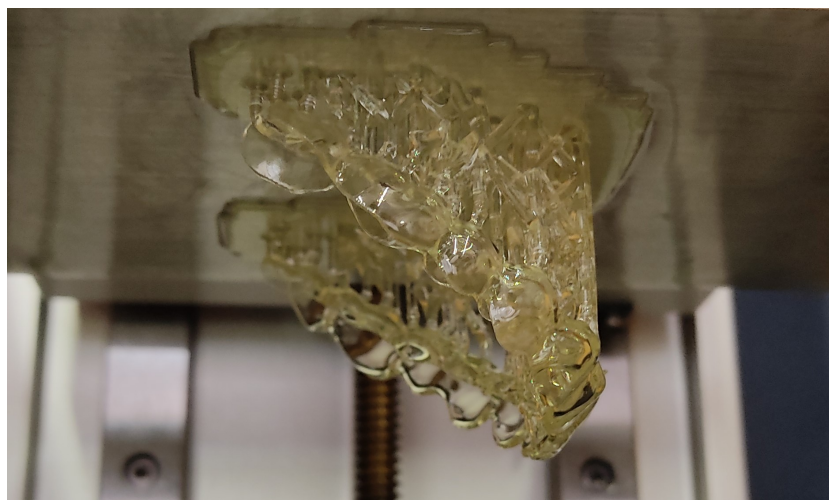
Figure 5. Result of direct printing DLP technology: the clear aligner with supports.
