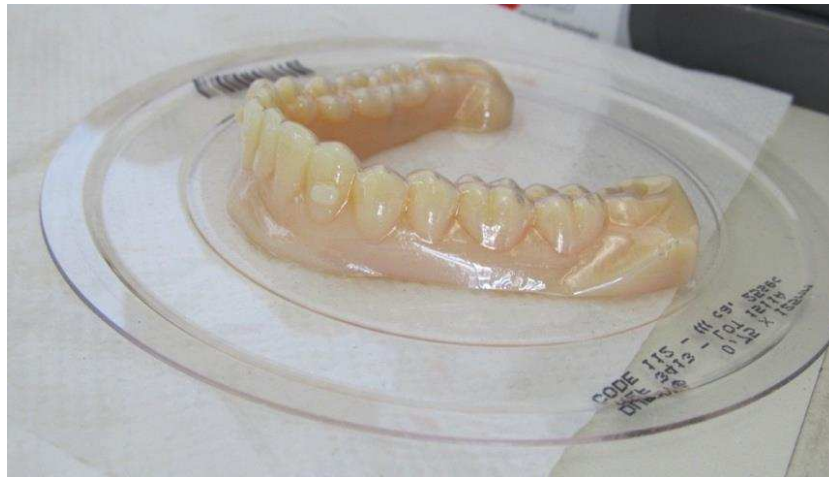
Figure 4. Results of the thermoforming process: aligner thermoformed on the printed model.
