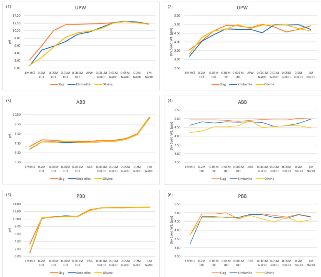
Figure 1. Change in pH (left) and change of mass of minerals after filtration (right) in different concentrations of acid (0.001, 0.01, 0.05, 0.2, and 1 mol/L), unaltered aqueous solution (UPW/ ABB/ PBB) and base (0.001, 0.01, 0.05, 0.2, and 1 mol/L) for EAF slag, olivine, and kimberlite in UPW, ABB and PBB.
