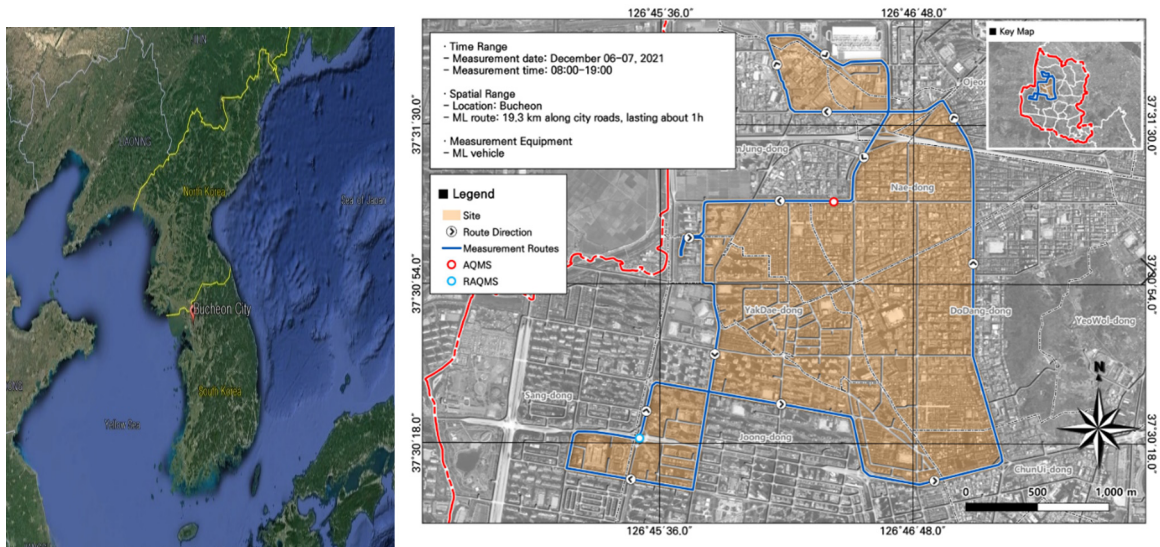
Figure 1. Location of the study site, mobile laboratory (ML) route, and fixed air quality monitoring system (AQMS) and roadside air quality monitoring system (RAQMS) stations.
