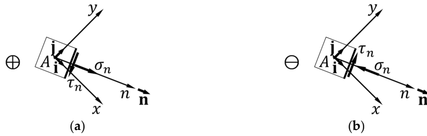
Figure A3. Stress components acting on the plane with unit normal vector \mathbf{n} (the plane perpendicular to the outward-pointing line n ) in the reference frame of Figure A1: (a) For normal and shear stresses that are positive in the Mohr plane; (b) For normal and shear stresses that are negative in the Mohr plane.
