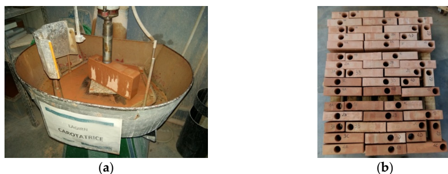
Figure 17. Preparatory stages for laying bricks: (a) Core drilling of a brick; (b) Drying of bricks after core drilling.
