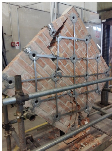
Figure 27. Failure mode of Specimen M2-45.
