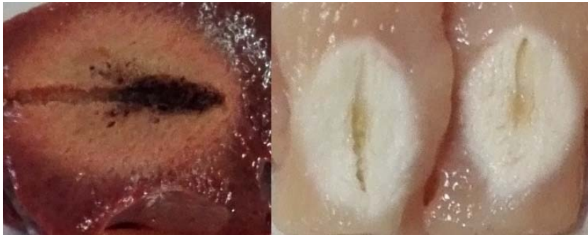
Figure 8. Example of ablation in bovine liver (left) and chicken breast (right).
