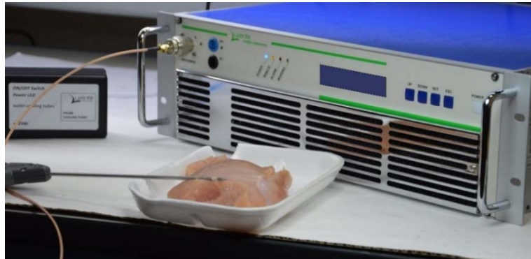
Figure 3. Hybrid dual frequency MW+RF generator in an experimental setup for MWA performed on chicken breast
