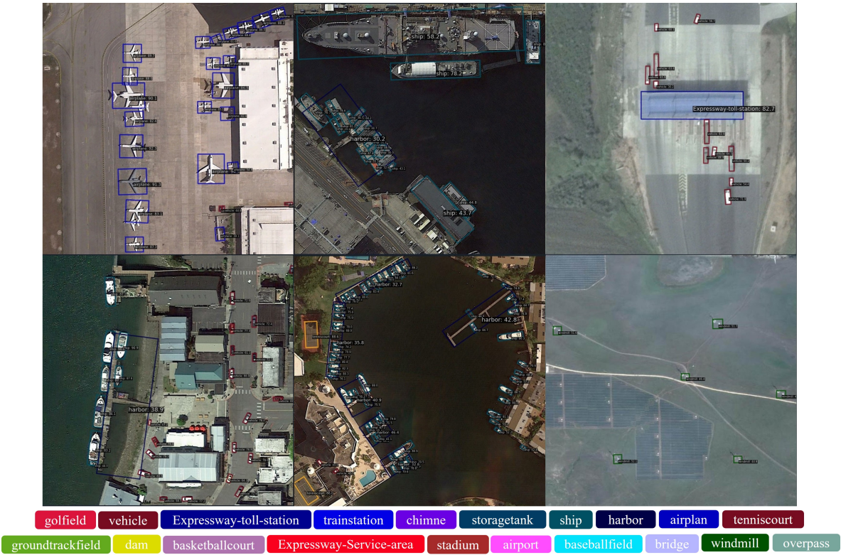
Figure 5. Here are some detection results of our proposed MFCA model on DIOR-R. Each color represents a distinct category, and the displayed results include six classes: ships, harbors, airplanes, vehicles, windmills, and expressway toll stations. It is evident that the MFCA module excels at identifying dense small targets amidst complex backgrounds.
